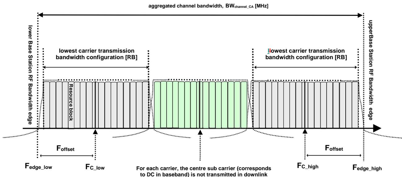
**Figure 3.1-2: Aggregated Channel Bandwidth for intra-band carrier aggregation**
